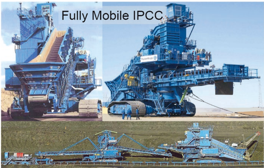
Fig. 3.10 Fully mobile IPCC (Koehler 2010)
