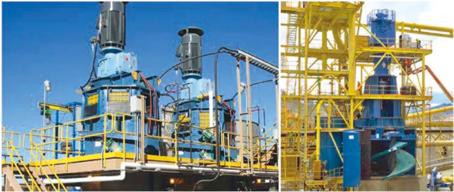
Fig. 4.5 Industrial Vertimill (Allen 2013; Lakshmanan et al. 2016)
