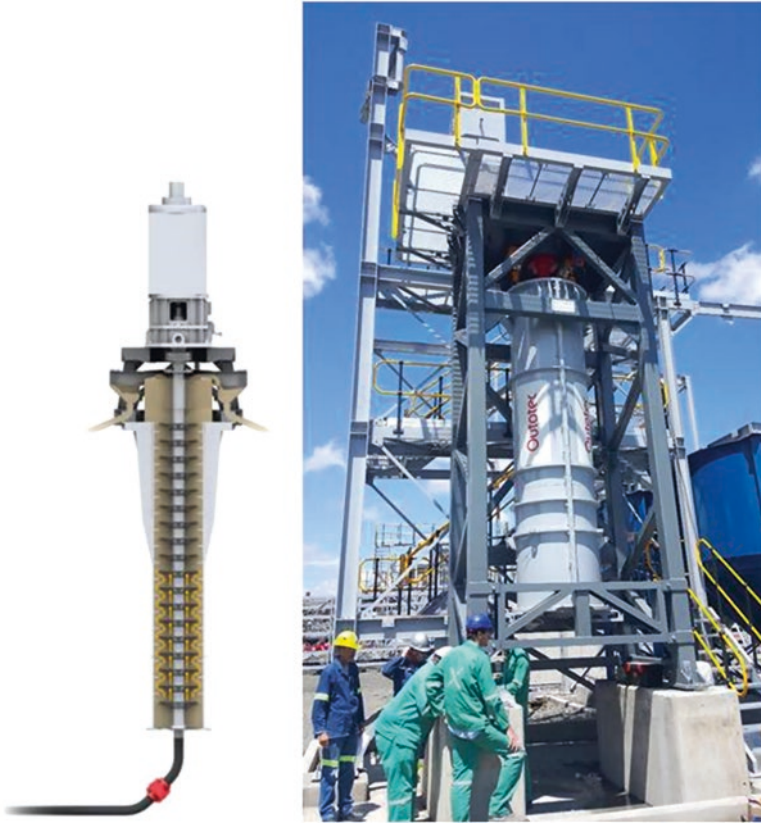
Fig. 4.8 Outotec industrial HIGmill (Letho et al. 2013)
