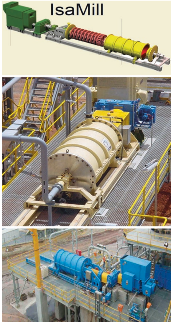
Fig. 4.3 Industrial IsaMill (Glencore 2015)
