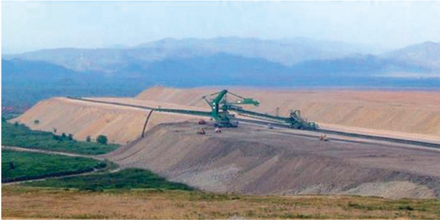
Fig. 3.9 Semi-mobile IPCC system (Courtesy of Sandvik) (Johnson Marc 2014)
