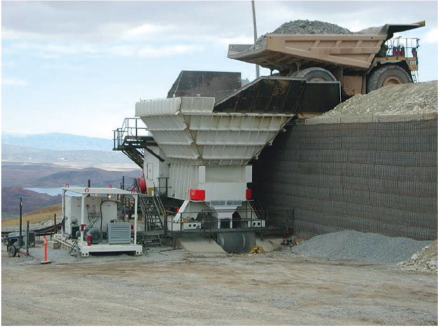
Fig. 3.7 Fixed IPCC system (Szalanski Scot 2009)
