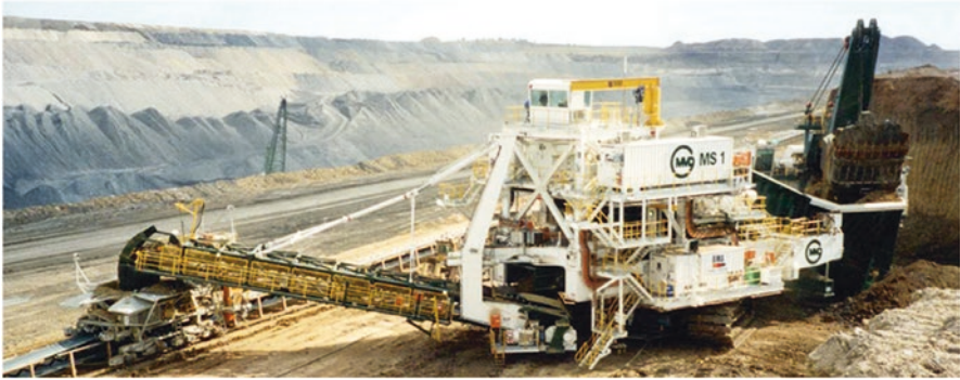
Fig. 3.11 Fully mobile sizer (Crusher) (Courtesy of MMD) (Johnson Marc 2014)
