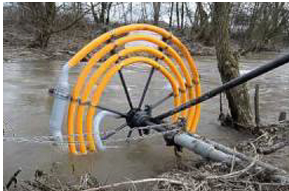
Fig. 6. Water wheel pumps
