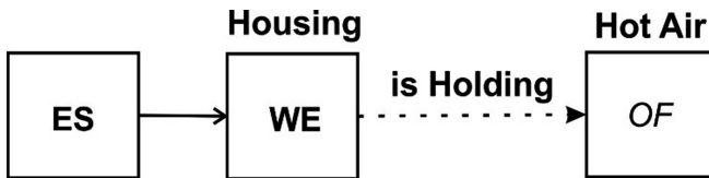
Fig. 5. Graphic representation of the element-functional model of conflict (EFM.C) [8]; where: ES – Energy Source; WE – Working Element; OF – Object of Function.
