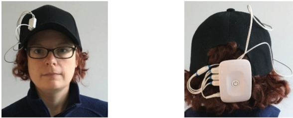
Fig. 1. Our commercial (TRL 8), ruggedized, field-ready fNIRS Pioneer TM (left)
