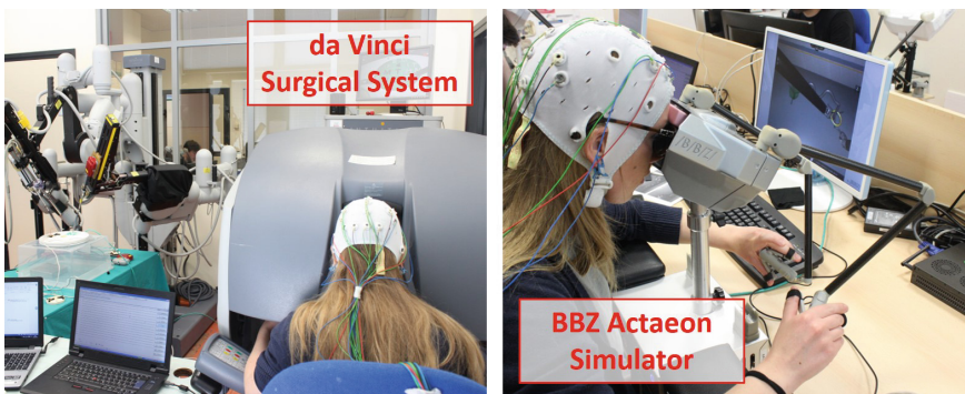
Fig. 1. The same student during the experiments performing the experimental tasks by the da Vinci Surgical System (on the left) and by the BBZ Actaeon Simulator (on the right).
