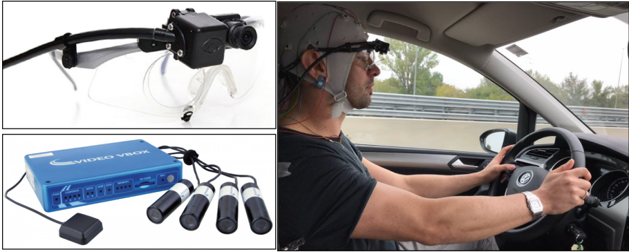
Fig. 3. ASL Mobile Eye-XG device, Video Vbox Pro data recorder and the driver inside the car during the test.
