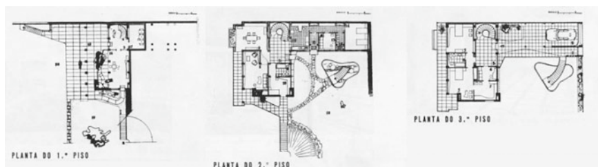
Fig. 4 “Moradia em Vila Nova de Gaia”, 3 floor levels in “L” shape. In Arquitectura , 2nd series, no. 44, 1952. Figures from the magazines, p. 4
