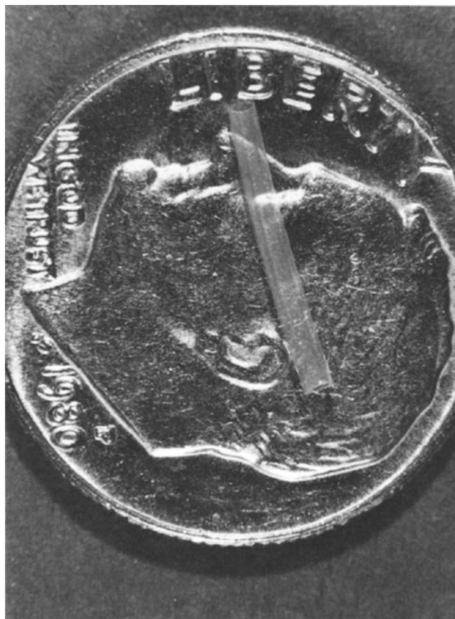
Fig. 15.1 Hollow polyglycolic acid stent (0.5-mm outer diameter) shown on a dime. (Used with permission from Flam et al. [30]. With permission from Elsevier)
