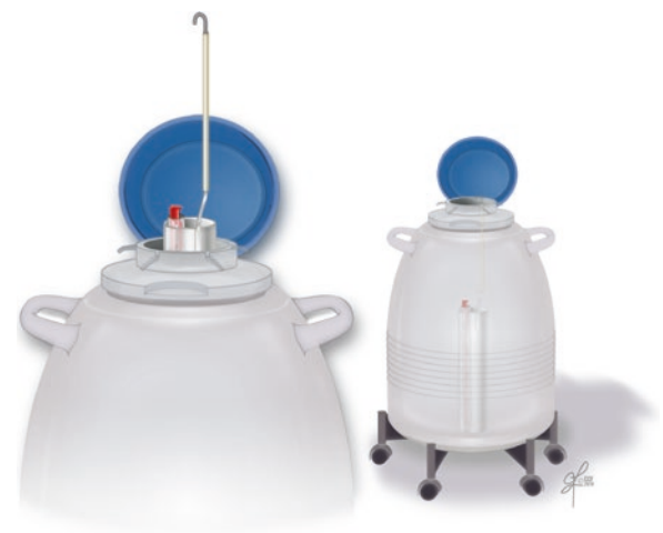
Fig. 22.8 Cryotank canister containing cryocanes and cryovials added slowly, upright into cryotank. (Reprinted with permission, Cleveland Clinic Center for Medical Art & Photography © 2014–2019. All Rights Reserved)
