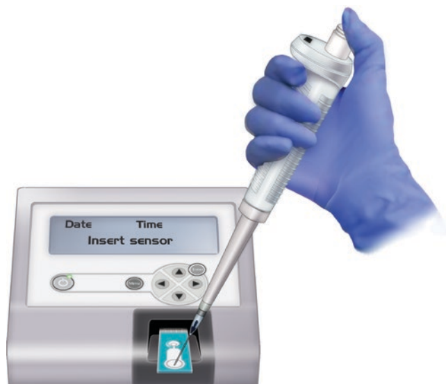
Fig. 7.11 A 30 \mu\text{L} sample is carefully aspirated and loaded on the sensor sample port. (Reprinted with permission, Cleveland Clinic Center for Medical Art & Photography © 2013–2019. All Rights Reserved)
