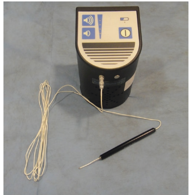
Fig. 4.1 VTI surgical Doppler 9.3 MHz and a disposable probe flow detector (Vascular Technology Int., USA)
