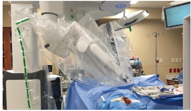
Fig. 19.3 Positioning of the robotic system at a 90° angle to the patient with the camera positioned directly above the operative field (view from console)
