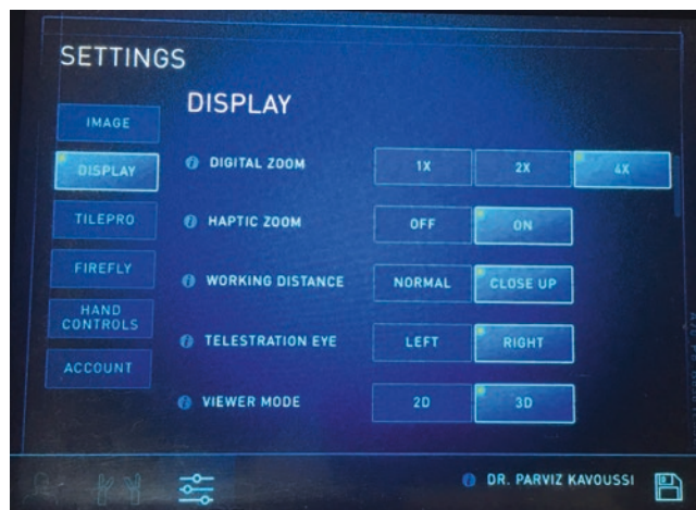
Fig. 19.7 Robotic platform settings including a 4× digital zoom, haptic zoom, a close-up working distance setting, and a three-dimensional viewer mode
