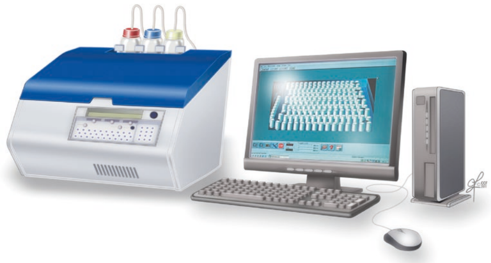
Fig. 7.2 Autolumat 953 Plus Luminometer used in the measurement of ROS by chemiluminescence assay. Multiple tubes can be loaded simultaneously for measuring ROS. The luminometer can be connected with a computer and monitor. (Reprinted with permission, Cleveland Clinic Center for Medical Art & Photography © 2013–2019. All Rights Reserved)
