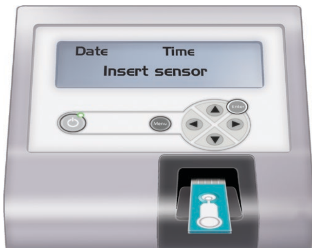
Fig. 7.10 The MiOXSYS Analyzer is turned on and the sensor is gently placed on the sensor module. (Reprinted with permission, Cleveland Clinic Center for Medical Art & Photography © 2013–2019. All Rights Reserved)
