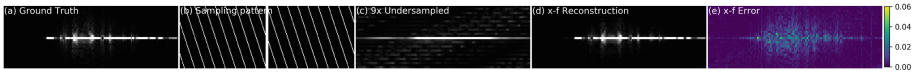
Fig. 3. Visualisation in x-f domain. (a) Ground Truth (b) k-t sampling pattern (c) 9× undersampled data (d) Reconstructed x-f image (e) Error between (c) and (d).
