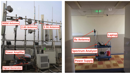
Fig. 1. The photos of the multi-band channel sounder. (a) TX System; (b) RX System
