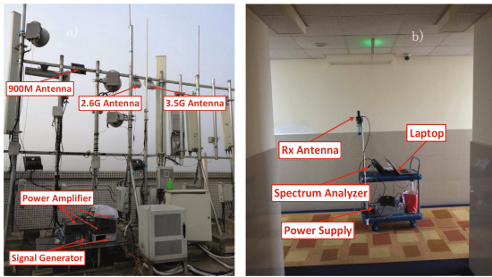
Fig. 1. The photos of the multi-band channel sounder. (a) TX System; (b) RX System
