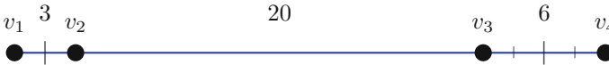
Fig. 10.4 Network of Example 10.4 where the dots, the ticks and the small ticks are the nodes, the equilibrium points and the elements of Y , respectively. Observe that in this case there are no pairs in T
