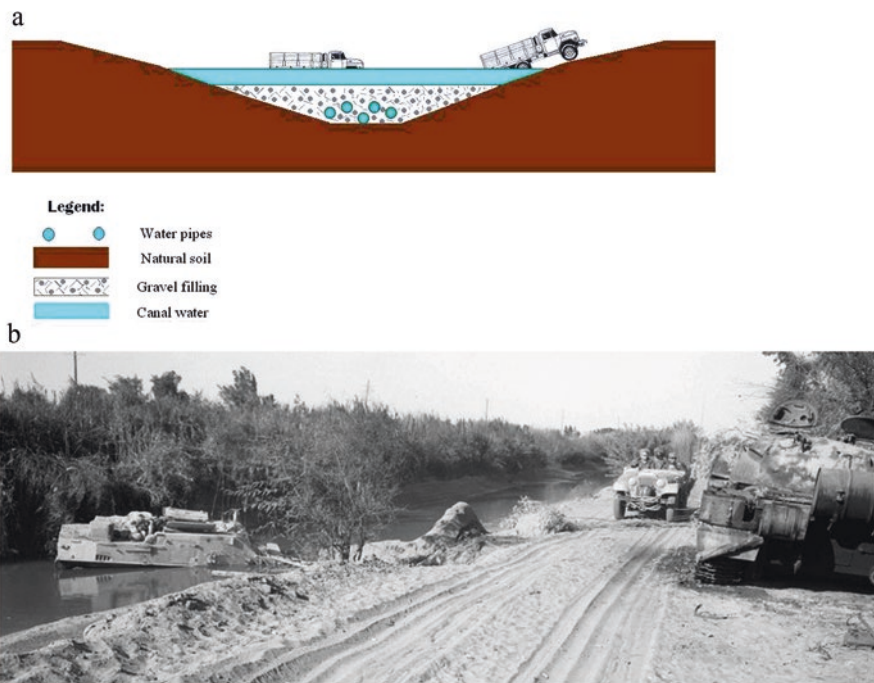
Fig. 10.3 The Sweet Water Canal. (a) Sketch of a submerged underwater passage made of gravel, (b) Egyptian armored personnel carrier stuck on a submerged passage. (Photo by E.D)
