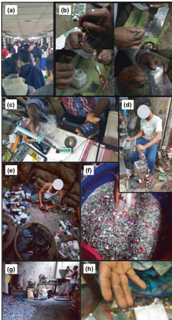
Fig. 11.1 E-waste repair/recycling in Bangladesh: (a) underground market for electronics repair, (b) electronics repair with bare hands, (c) fume-exposure during electronics repair, (d, e) separating Fig. 11.1 (continued) and sort of recyclable metals, plastics, wires, etc. using bare hands, (f) plastic washing with water, (g) plastic melting to produce beads, and (h) worker's hand with skin lesions. (Source: Compilation of photos from author: Syed Ishtiaque Ahmed)
