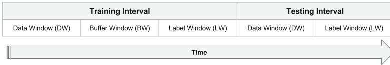
Fig. 1. Overview of a Classification Exercise (CE). Each exercise is divided into two broad phases: training , during which the classifier is fitted, and testing , during which the classifier predictions are evaluated. Each phase is subdivided into smaller non-overlapping time windows: Data Window (DW), Buffer Window (BW) and Label Window (LW). The DW is the period of time over which behavioural features are mined. The BW is a period of time introduced to avoid learning from accounts that may already be compromised but not yet labeled as such. The LW is the period over which labels are extracted.
