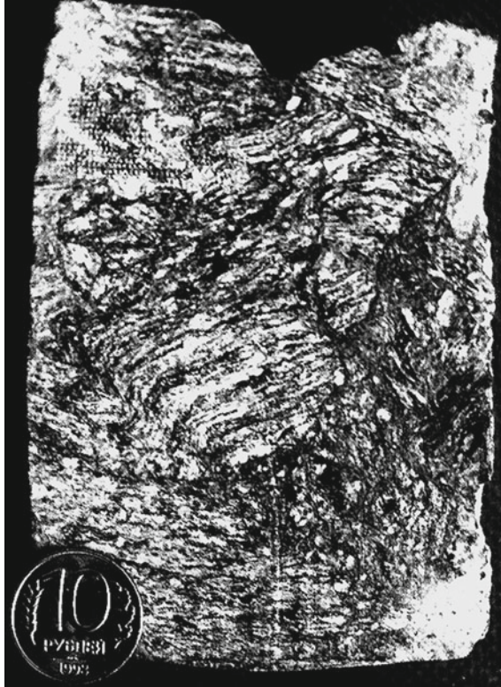
Fig. 18 Cataclasite after amphibole-biotite gneiss composed of fragments rumbled to a variable extent and cemented by fine-granular polymineral matrix (dark) (VDW, depth 920 m). Natural size
