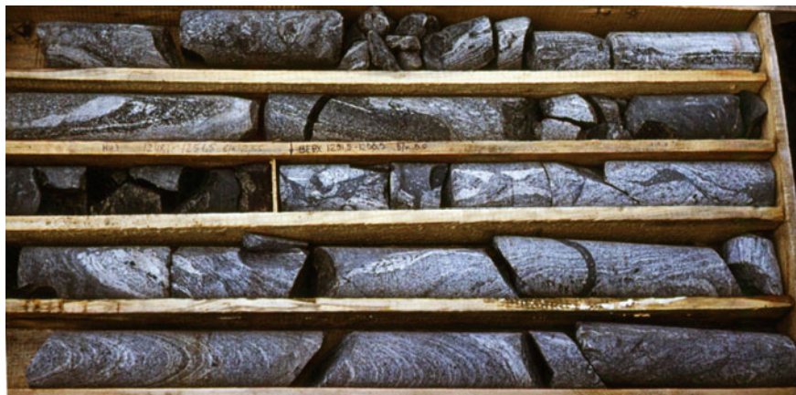
Fig. 21 Brecciated and cataclased shocked amphibole-biotite gneiss with thin tagamite veins. VDW, depth 1250.5–1255.5 m. Core diameter is 73 mm
