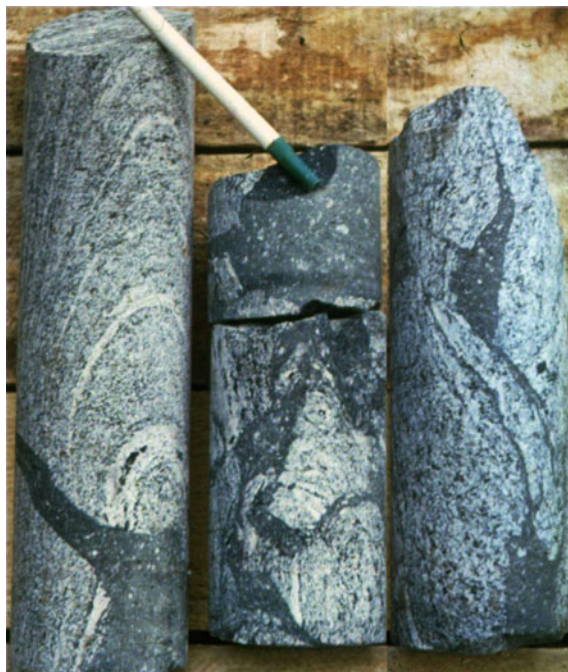
Fig. 35 Thin veins (no more than 3 cm thick) and spots of tagamite in shocked gneiss. VDW core, depth 1250–1251 m. Core diameter is 73 mm
