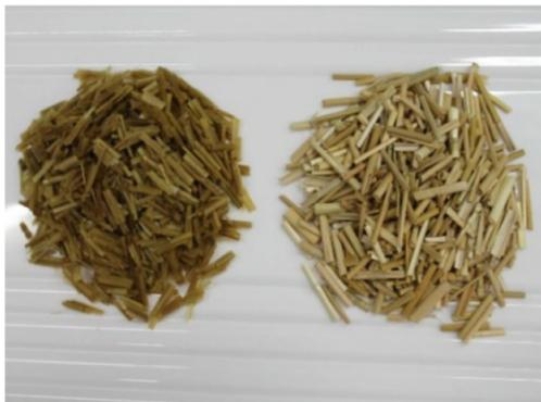
**Fig. 2.** Wheat straw additive before (right-hand side) and after (left-hand side) the treatment
