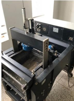
Fig. 8. Large-scale direct shear apparatus (Geocomp ShearTrac III)
