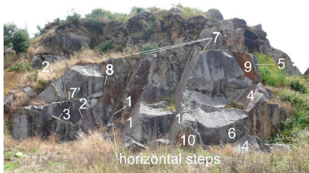
Fig. 2. Identification of the discontinuity sets identified during the fieldwork.
