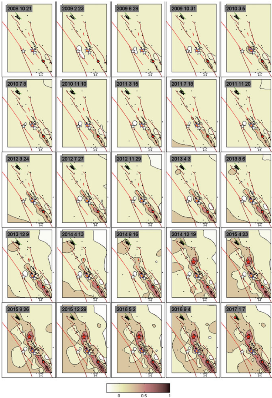
Fig. 2 Spatiotemporal distribution of total shear deformation. Isolines are drawn through 0.25 \cdot 10^{-5} . The big red star is the Napa earthquake M = 6.0 . Small white stars are the strongest historical earthquakes. A small orange star is an expected catastrophic earthquake [4, 5]. Red circles are moderate earthquakes M = 5.4-5.6 . Black dots are small earthquakes 3 < M < 5 . For the legend of faults, see Fig. 1
