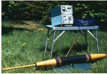
Fig. 2 Search-coil magnetometer INT-1 for recording geomagnetic pulsations
