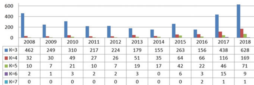
Fig. 2 Distribution of the seismic events by energy classes recorded in the Saamsky fault area for a 10-year monitoring period
