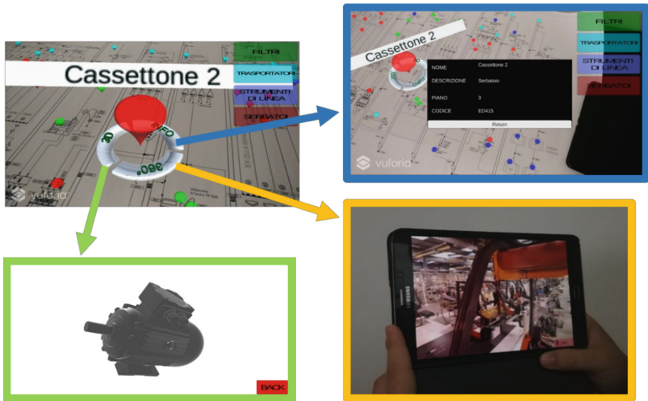
Fig. 2. Visualization of additional technical information through a pie menu: a technical chart with information retrieved from a database, a navigable 3D CAD model, and a 360-degree image of a plant section.
