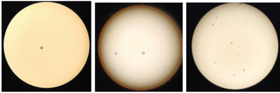
Fig. 6 The yeast fungus after it has gone through the decontamination system filled with quartz fibers during 10 min. The number of colonies after the mediation on 10 experiments was 1.5
