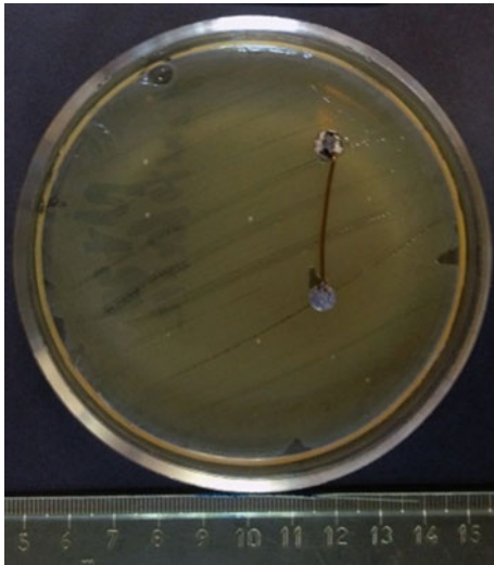
Fig. 4 The diameter of the growth retardation zone of Acinetobacter baumannii on agar under electrodes in a closed loop energy circulation
