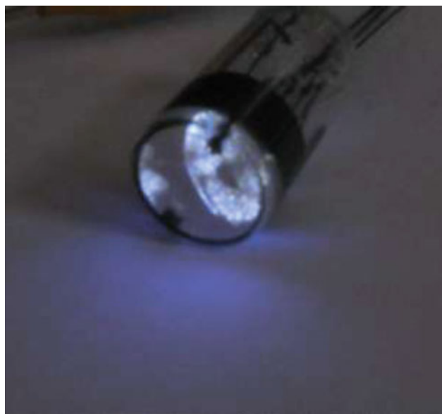
Fig. 1 Finger-type cathodoluminescent UV lamp (switched on)
