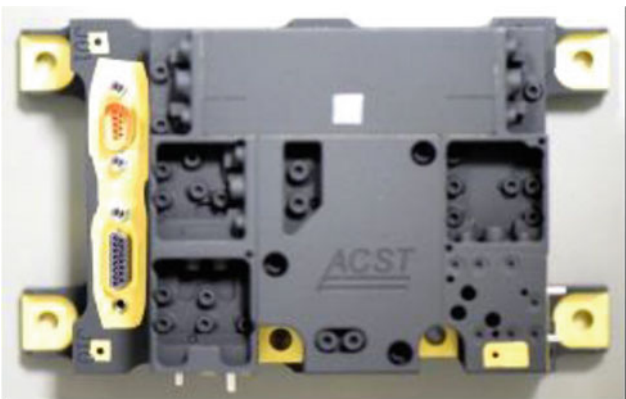
Fig. 3 DA-design 89 GHz EQM receiver with integrated ACST detector in the centre
