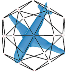
Fig. 2. Virtual cameras are placed at each vertex of a tetrahedron to render the 3D shape model.
