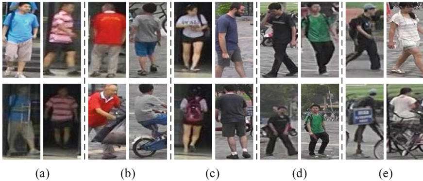
Fig. 1. Some image pairs from the Market1501 [1] dataset. The upper and lower adjacent images have the same identity: (a) variations in illumination. (b) variations in posture. (c) variations in viewpoint. (d) variations in misalignment. (e) variations in background occlusion.
