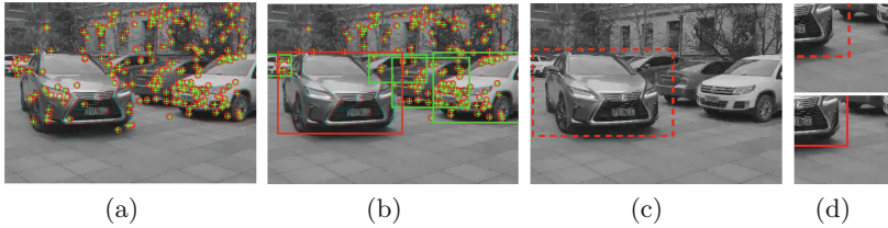
Fig. 7. Detection results and threat boxes (a) Match results of SURF (b) Results with YOLO detection and constrains, the moving car is marked by red box, static cars by green boxes (c) Constructed threat box for the moving car. (d) Detail comparison of YOLO detection and our threat box (Color figure online)
