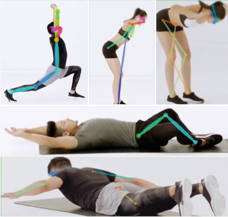
Fig. 1. Limitations of applying current pose estimation models on some workout postures, which have severe self-occlusion. Some body keypoints are falsely detected or missed in prediction even the background is plain.
