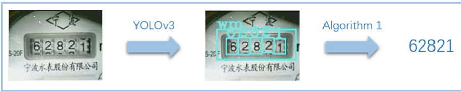
Fig. 5. Water meter recognition flowchart in this paper, YOLOv3 for RoIs regression and classification, then additional algorithm to solve half-word problem
