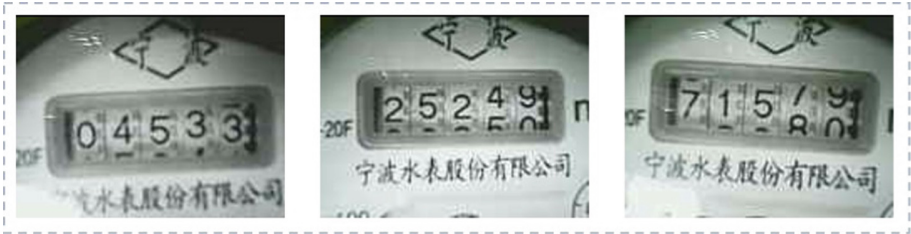
Fig. 1. The examples of water meter images. All the three sub-images have difficulty (1) and (2), the second and third sub-image significantly have difficulty (3) and (4).
