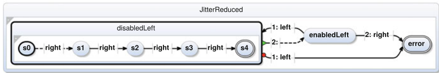
Fig. 10 Periodic behavior with jitter. (a) Automatically generated SCChart for jitter. (b) Simplified SCChart for jitter
