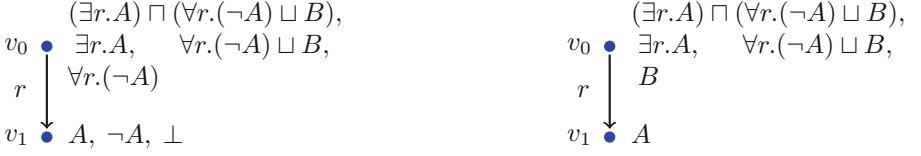
Fig. 2. Two possible tableau expansions for the concept C = (\exists r.A) \sqcap (\forall r.(\neg A) \sqcup B) due to the non-deterministic \sqcup -Rule
