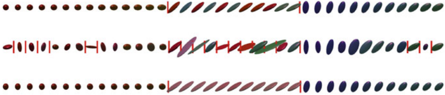
Fig. 2.8 Univariate Mumford-Shah regularization ( p, q = 1 ) using dynamic programming. (The red steaks indicate jumps.) Top. Original signal. Middle. Data with Rician noise added. Bottom. Regularized signal. Mumford-Shah regularization removes the noise while preserving the jump
