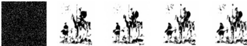
Fig. 7.7 Image inpainting from an image f with 95% missing pixels (left) by minimizing R(u) among images u : \Omega \rightarrow [0, 1] coinciding with f at the given pixels. Same regularizers, discretizations and parameters as in 7.6
