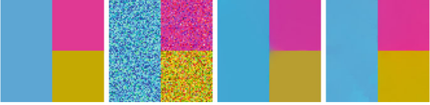
Fig. 2.1 The effect of \ell^2 -TV denoising in LCh space ( \alpha = 0.80 ). Left. Ground truth. Middle left. Noisy input image corrupted by Gaussian noise on each channel. Middle right. The \ell^2 -TV reconstruction in linear space. Right. The \ell^2 -TV reconstruction in the nonlinear LCh color space. Using the distance in the non-flat LCh metric can lead to higher reconstruction quality
