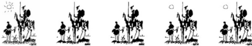
Fig. 7.6 Binary segmentation of an image f : \Omega \rightarrow [0, 1] (left) by minimizing \lambda \int_{\Omega} (\frac{1}{2} - f)u_x + R(u) among images u : \Omega \rightarrow [0, 1] with regularizer R chosen as R_{\rho_0} (second, using finite differences, and third, using adaptive line measure segments), as R_2 with g(\kappa) = \kappa^2 (third, using curved line measure segments), and as R_3 with g(\kappa) = \kappa^2 (right, using Raviart–Thomas Finite Elements). In all experiments \Omega = [0, 1]^2 , \beta = 1 , \alpha = 25 , \lambda = 256^2
