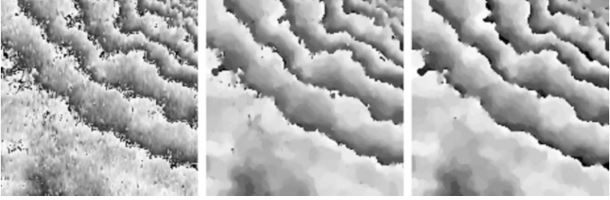
Fig. 2.4 Total variation denoising of an \mathbb{S}^1 -valued InSAR image (real data, left ) using L^2 -TV regularization ( \alpha = 0.32 , middle ) and L^1 -TV regularization ( \alpha = 0.60 , right ). Here, the circle \mathbb{S}^1 is represented as an interval with endpoints identified, i.e., white and black represent points nearby. Total variation minimization reliably removes the noise while preserving the structure of the image
