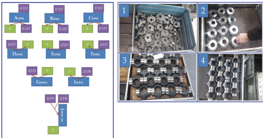
Fig. 7. The contents and location of pallets after the first working shift and the “Swinging plate” component in individual stages of the production process
