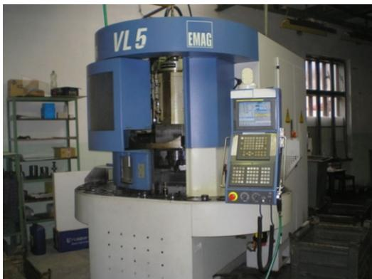
**Fig. 1.** Vertical turning machine for hard turning
