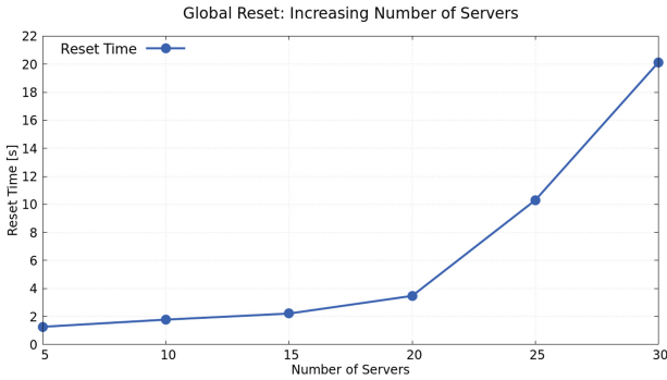
Fig. 4. The time it takes for the Global Reset mechanism to complete, with respect to the number of servers.
