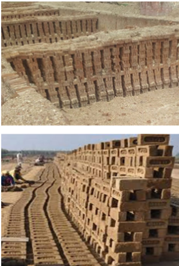
Fig. 13.3 Brick making with clay in Begusarai and Bhagalpur, Bihar
