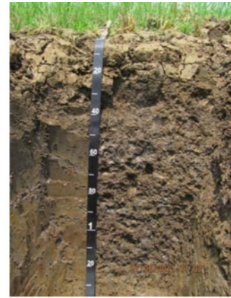
Soils of Typic Endoaquents in flood plains of Eastern region (West Bengal)
