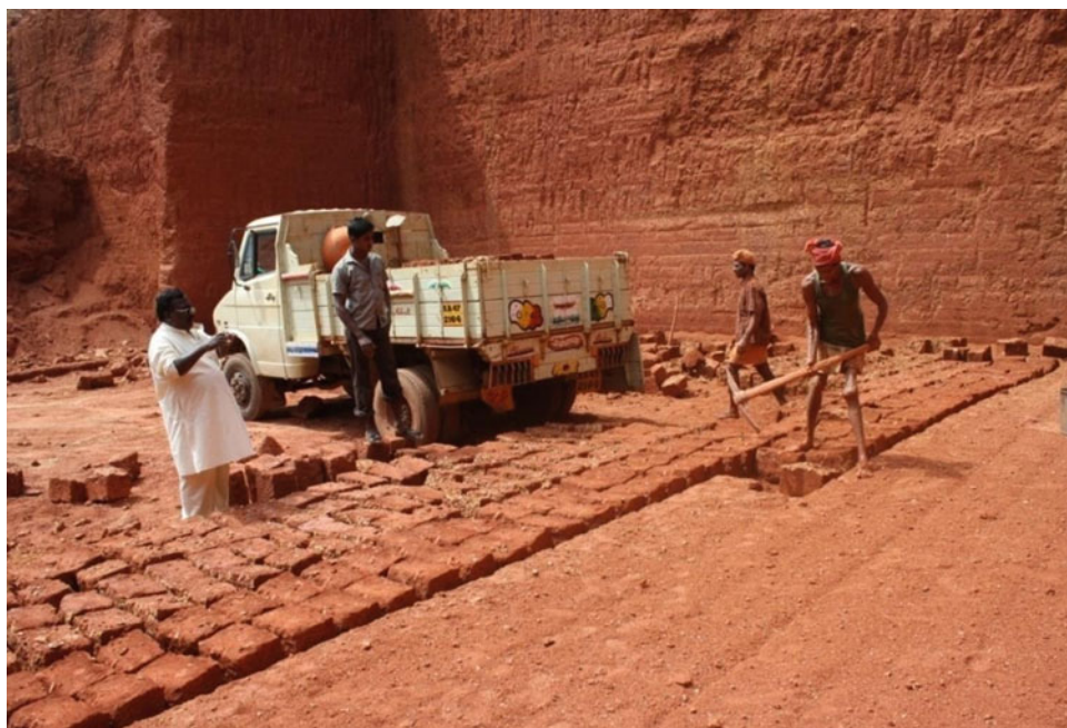
Fig. 4.6 Laterite brick cutting at Kumta, Udupi district, Karnataka Catenary sequence of lateritic terrain of Karnataka plateau. Source NBSS&LUP Archives 2017
