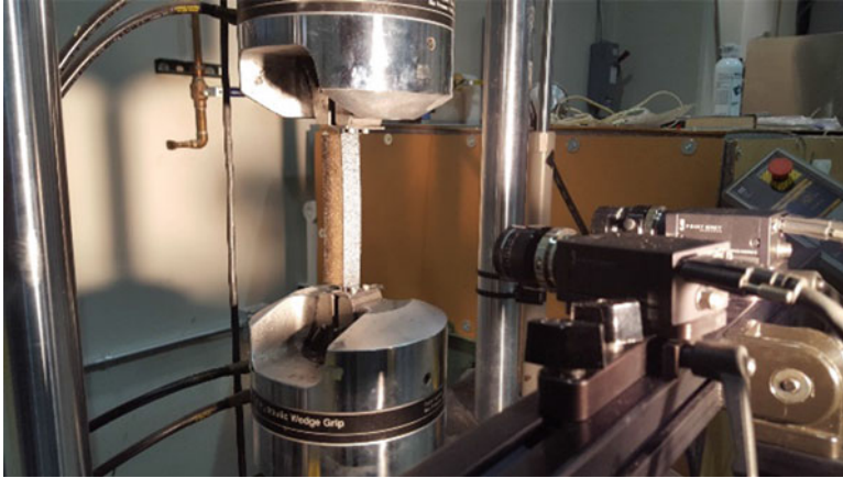
Fig. 22 Experimental set-up with dry matrix dominated CFVE sandwich specimen
