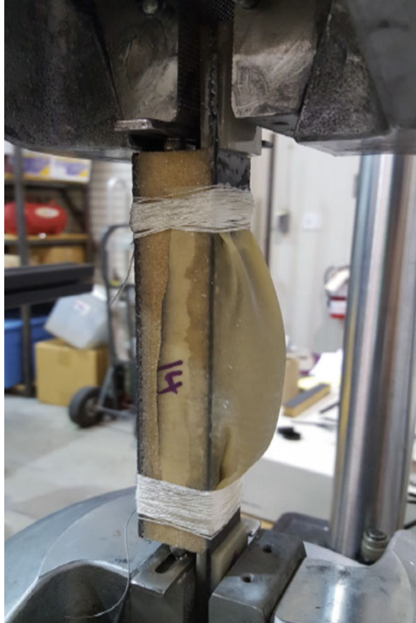
Fig. 23 Matrix dominated wet CFVE specimen with one-sided water confinement
