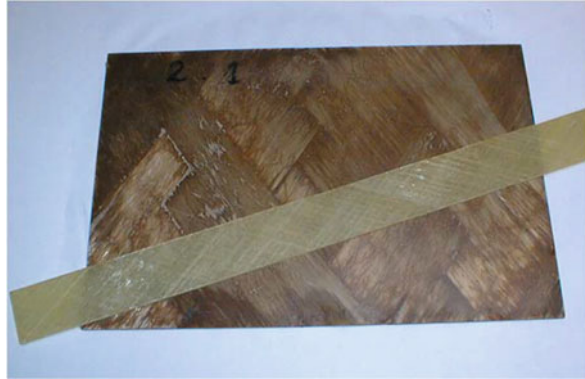
Fig. 17 Weight gain panel (200 × 300 mm 2 ) after 7.7 years in distilled water at 60 °C, and unaged reference strip
