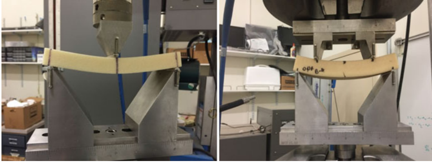
Fig. 1 (Left) three-point bending test on PU foam; (right) four-point bending test on PVC foam
