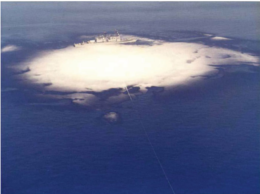
Fig. 5 Bulk cavitation at the sea surface from an underwater explosion [4]
