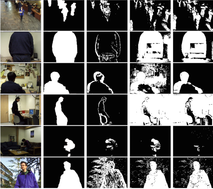
Fig. 3. Qualitative results. From left to right: original image, ground truth, Frame Difference, GMM1, GMM2. From top to bottom: bootstrap (BS), camouflage (CA), foreground aperture (FA), lightswitch (LS), time of day (TD), waving trees (WT).
