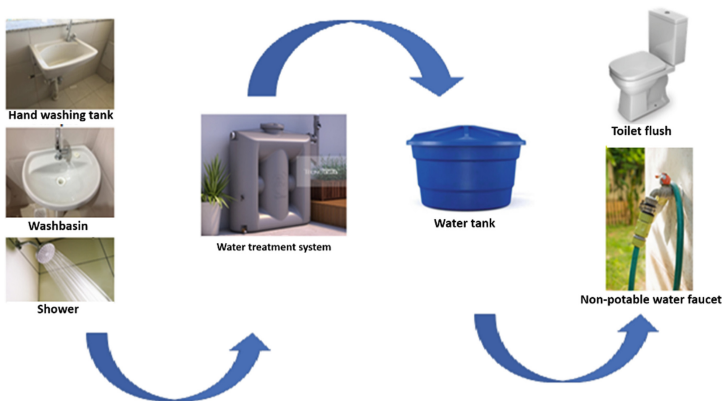
Fig. 2. Flowchart of the greywater treatment and reuse system. (Source: the authors, 2017)
