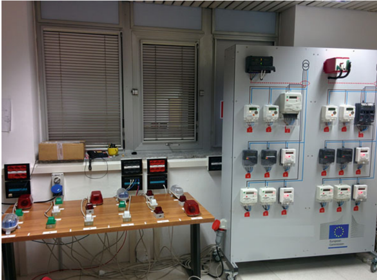
Fig. 6 The smart meter infrastructure setup
