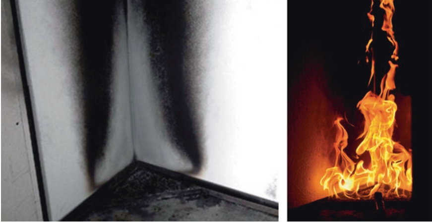
Fig. 23.20 Implementation of fire tests single burning item (SBI) at IBS—Institute for Fire Protection and Safety Research [3]
