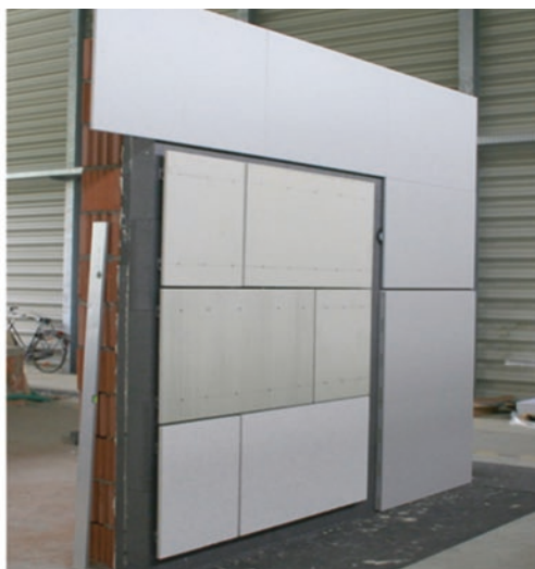
Fig. 23.25 Weather independent assembly tested winter -10\text{ }^{\circ}\text{C} [3]
