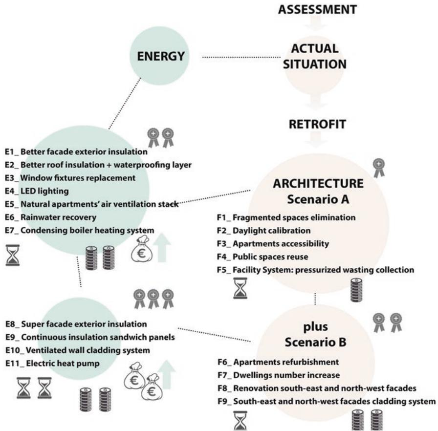
Fig. 16.4 Design solutions diagrams and energy retrofit actions
