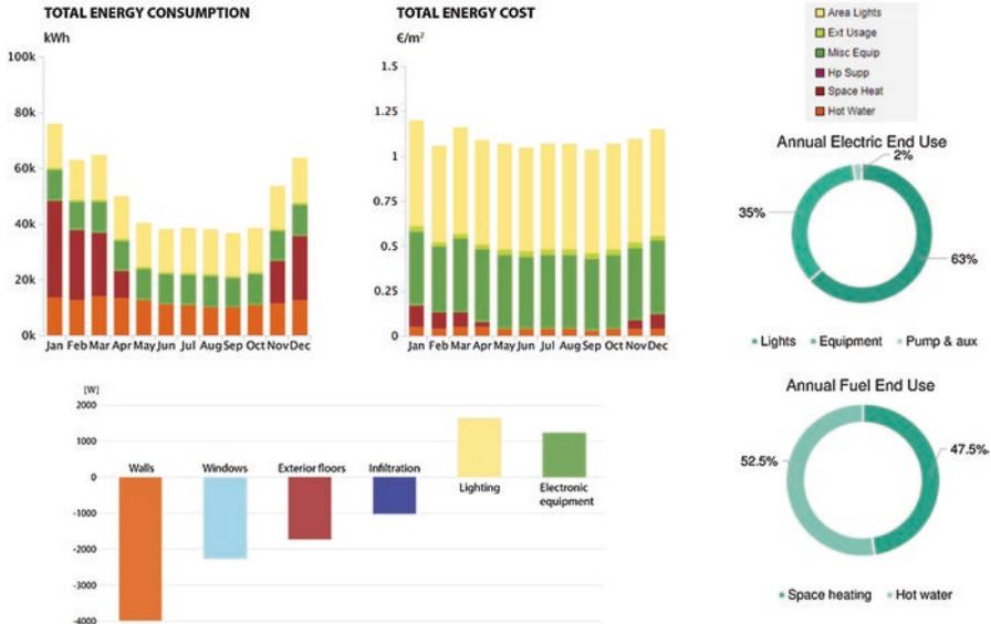
**Fig. 16.8** Results of the dynamic analysis for the actual situation: total energy consumption and total energy cost (top-left), energy consumption in terms of electric energy and natural gas fuel (right) and heating load analysis of building components (bottom-left)
