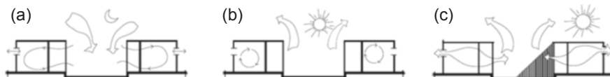
Fig. 12.2 Air circulation between the courtyard and adjoining rooms at night (a), midday (b) and afternoon (c). (Source: adapted from [3], p. 108)
