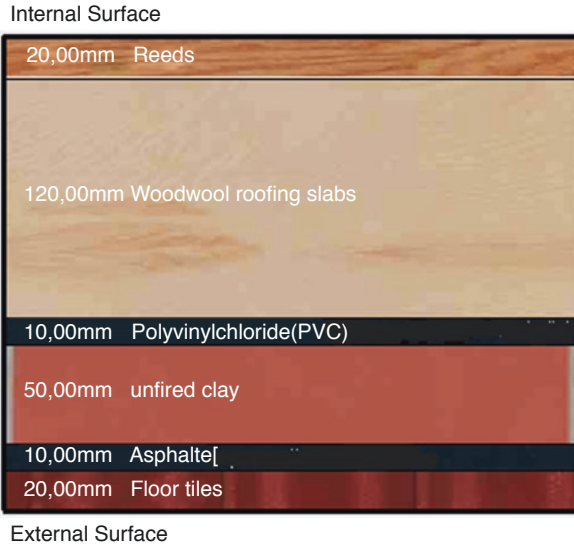
Fig. 24.6 External roof layers
