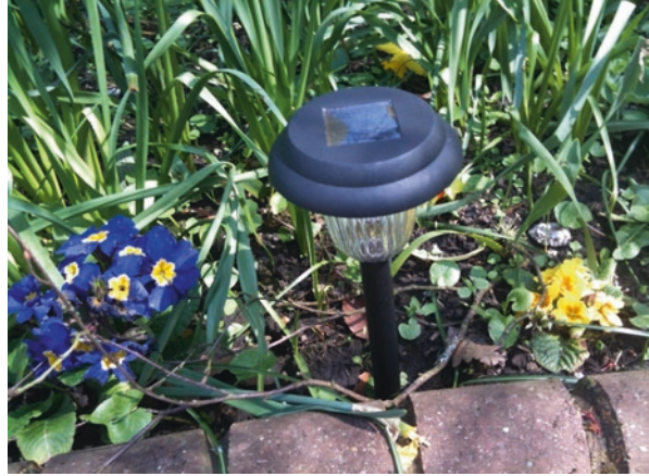
Fig. 43.7 A stand-alone garden lantern with no mains connection needs battery storage
