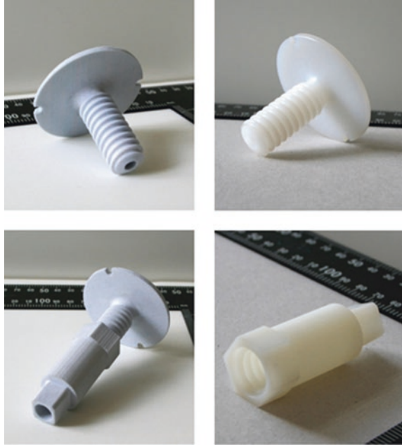
Fig. 23.11 Prototypes manufacturing techniques of mechanical fixation: laser sintering, laminated object modelling and CNC milling [3]
