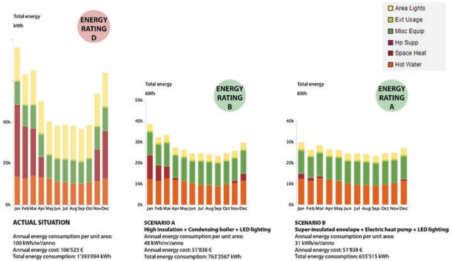
Fig. 16.10 Energy ratings and energy consumptions for actual situation (left), scenario A (centre) and scenario B (right)
