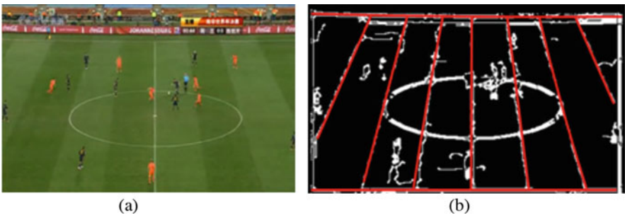
Fig. 3 Features extraction of stadium line. (a) Original image, (b) Extracted field line
