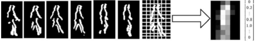
Fig. 2 Contour sequence and block feature representation of a player
