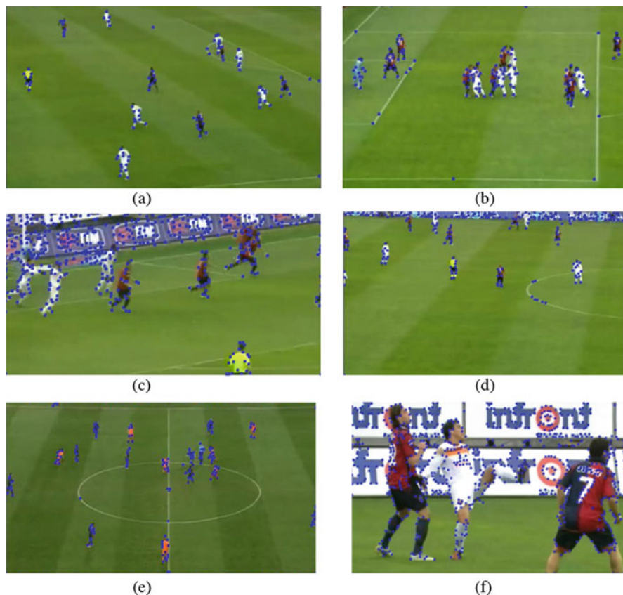
Fig. 6 Detection results of temporal and spatial interest points. (a) 52nd frame, (b) 88th frame, (c) 137th frame, (d) 223rd frame, (e) 76th frame (another video), (f) 361st frame (close-up frames)
