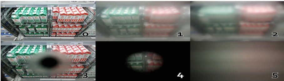
Fig. 1. Vision impairments simulated with mock optics. 0 - Full vision. 1 - Diabetic retinopathy. 2 - Cataract. 3 - Age-related macular degeneration (AMD). 4 - Narrow field of view i.e. retinitis pigmentosa (RP). 5 - Only light vision
