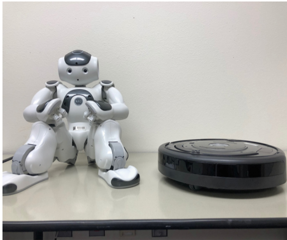
Fig. 1. NAO Robot (anthropomorphic) on the left and iRobot (mechanomorphic) on the right
