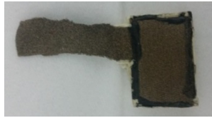
Fig. 2. Textile electrode built based on conductive fabric MedTex™ P-180.
