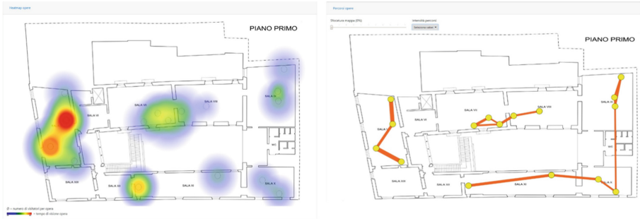
Fig. 6. An example of data visualization, where a heat map is used to demonstrate the behavior of the visitors.
