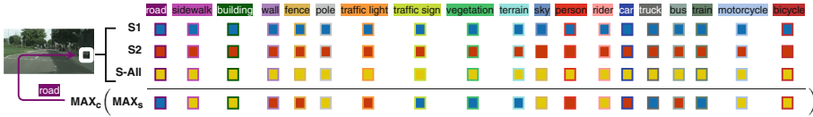
Fig. 2. Test Phase: each classifier produces a semantic segmentation output ( S1 : blue, S2 : red, S-All : yellow). For every pixel we apply a max-pooling operator over the three outputs. Finally the class assigned to the pixel is the one with the highest score over the C classes ( C = 19 when testing on Cityscapes). (Color figure online)
