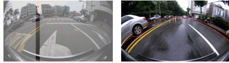
Fig. 3. Bottom point. Left: column-wise bottom prediction (red dot), Right: free space detection (red line). (Color figure online)
