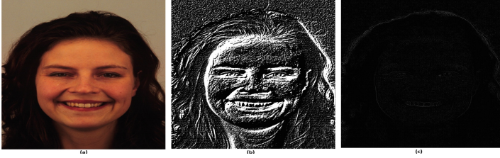
Fig. 2. (a) A sample input image from the KDEF dataset [23]. (b) Its derivative image obtained by the Sobel operator (Gradient). (c) Its second derivative obtained by the Laplacian operator. Zoom to see the details in the Laplacian image.
