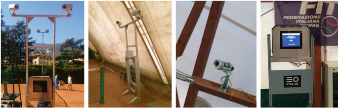
Fig. 5. System installed at CT Trento court without and with covering. Camera on the timber joists at CT Arco, and cabinet at CPO Tirrenia.
