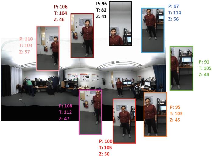
Fig. 2. The image shows an equirectangular image and a set of views acquired by different vPTZ cameras with the reported parameters.
