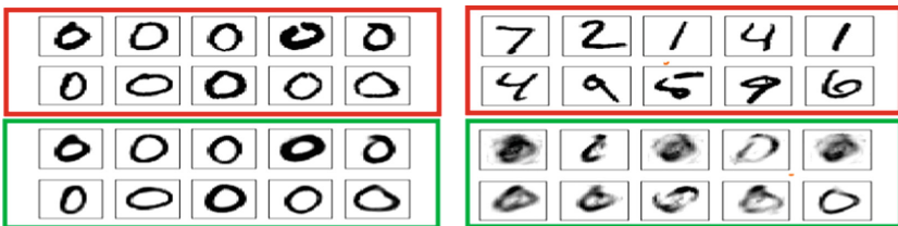
Fig. 4. Top rows: normal (left) and anomalous (right) samples from the MNIST test set. Bottom rows: the reconstructed images.
