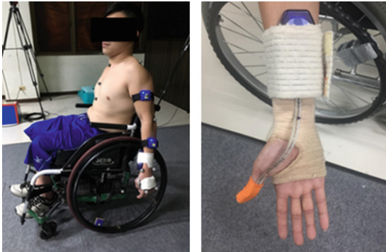
Fig. 2. Marker and sensor attachment on wheelchair and volunteers' upper limbs
