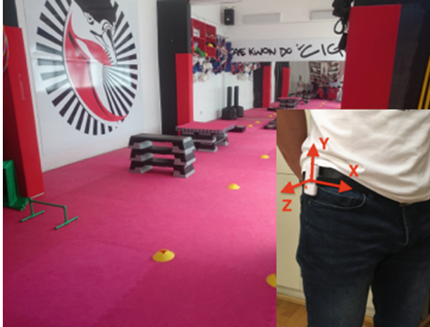
Fig. 1. Experimental setup for FER datasets. Subjects wore sensors attached to their waist and performed a set of ADL and simulated falls on a tatami mat.
