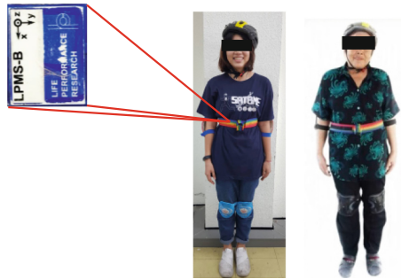
Fig. 1. Inertia sensor [5] orientation and placement on volunteers’s body
