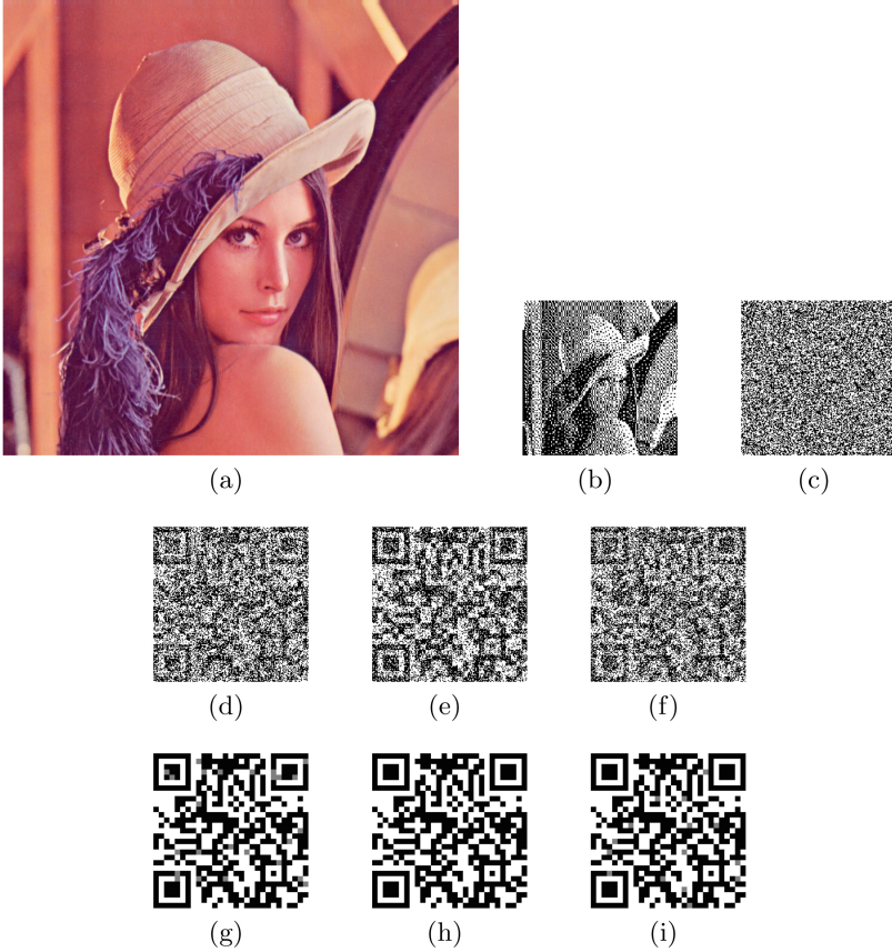
Fig. 6. Example results for the ‘lena’ image (a) input image; (b) dithered LL_2 sub-band; (c) visual depiction of the verification string; (d) S_R after JPEG compression; (e) S_R after noise; (f) S_R after blurring; (g) reconstructed QR code from (d); (h) reconstructed QR code from (e); (i) reconstructed QR code from (f).
