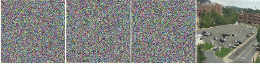
Fig. 4. Decrypted keyframes with incorrect keys (differ by a tiny value)
