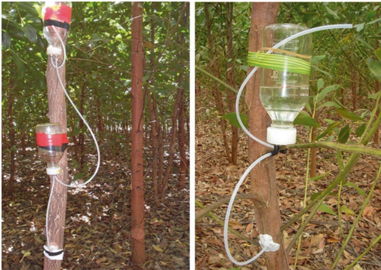
Fig. 56.1 Flasks and tubing to deliver distilled water or an ^{15}\text{N} solution to the xylem of trees selected for ^{15}\text{N} -labelling by the stem-injection method. Photos: R.R. Paula (left) and B. Zeller (right)
