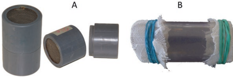
Fig. 51.2 Small enclosures made of PVC tubes to deploy invertebrates supplied with food to measure ingestion and growth rates in field conditions. Mesh screens of a defined size cover both ends of the tubes. Note the thread to unscrew the tube in type A and rubber bands to hold the loose mesh screens in place in type B
