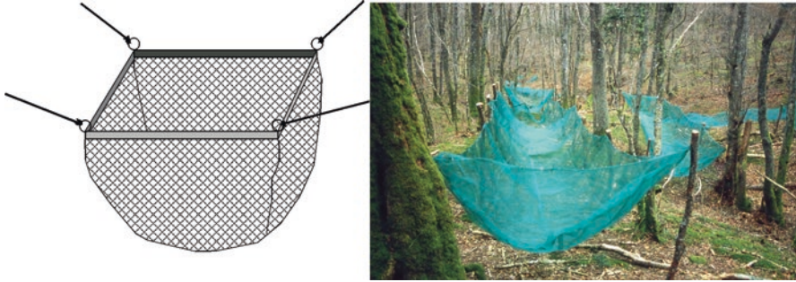
Fig. 1.1 (Left) A trap for determining vertical litter inputs. The mesh is fixed to a wooden or metallic frame hanging from nearby trees by four ropes. (Right) Three large traps set up in the riparian area and covering the total surface of the reach where inputs are estimated. The stream is further to the right, not visible on the photo
