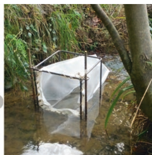
Fig. 1.3 (Left) Schematic of a typical drift net to sample CPOM in transport. The mesh is fixed to a metallic frame. Two metal rods can be used to secure the net in soft-bottom streams. A tube fixed at the end of the net makes sample collection easier. (Right) A modified version of the net shown in the drawing, deployed in a stream
