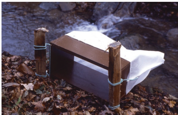
Fig. 1.2 A trap to determine lateral litter inputs to streams. The mesh is fixed to a wooden or metallic frame and secured to two stakes
