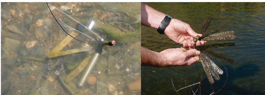
Fig. 8.1 Tongue depressors deployed (left) and recovered (right) from a river after 3 months of incubation. The shape has not changed, but they have suffered considerable mass loss
