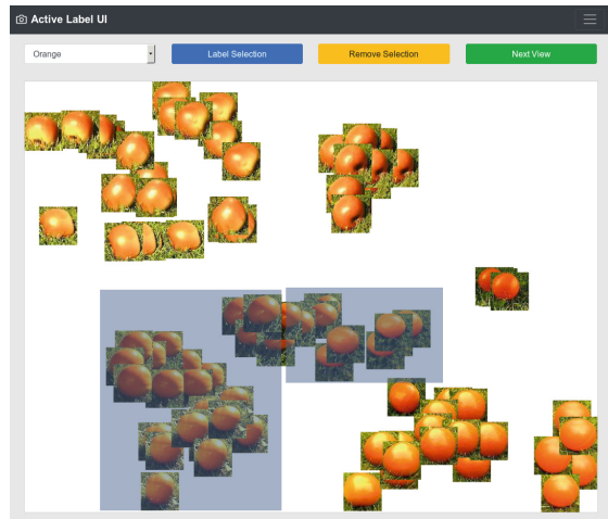
Fig. 3. Querying user interface showing a view queried by A2VQ. The user can label samples via selecting their thumbnails by dragging rectangles in the visualization. The class name can be entered in an input formula. With the button Label the selected samples are labeled and removed from the view. The button Remove Selection removes the rectangles. There are certain possible labeling strategies, like label everything, label only the biggest clusters or label only outliers. With a click on the button Query next view the classifier is retrained with the new labeled samples and a new view is queried with A2VQ.
