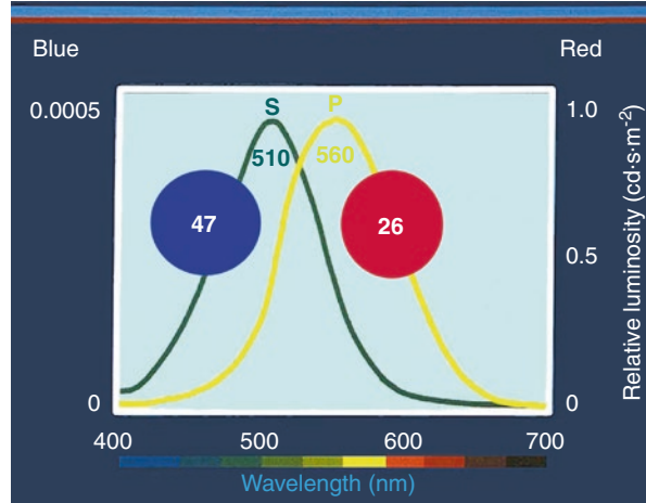
Fig. 1.6 Visual spectrum of 450 nm dim blue and above 580 nm dim red light flashes in relation to sensitivity curves of rods and cones showing example Wratten color filters used at dim flash intensities to isolate rod and cone physiology
